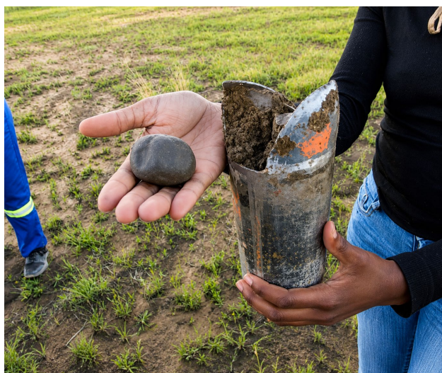
Figure 3. Soil samples collected from different soil forms: (a) high clay content and (b) texture observed through soil-profile horizons.
