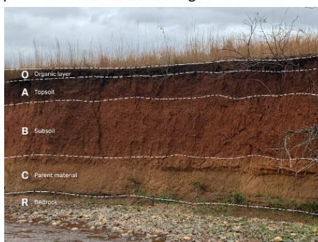
Figure 1. Example of in-situ soil classification in (b) eMlondozi, Mpumalanga.
