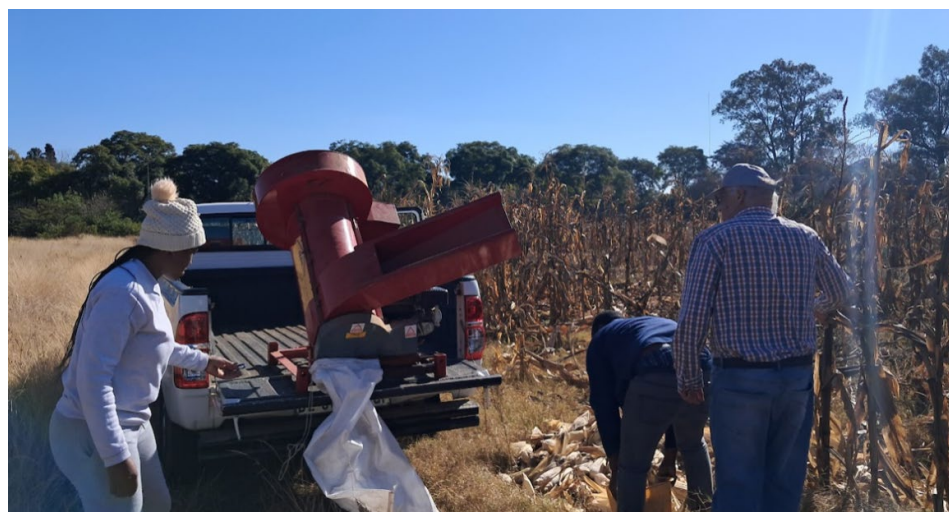
Figure 3: Agricultural Research Council staff testing a locally available thresher in the field.
